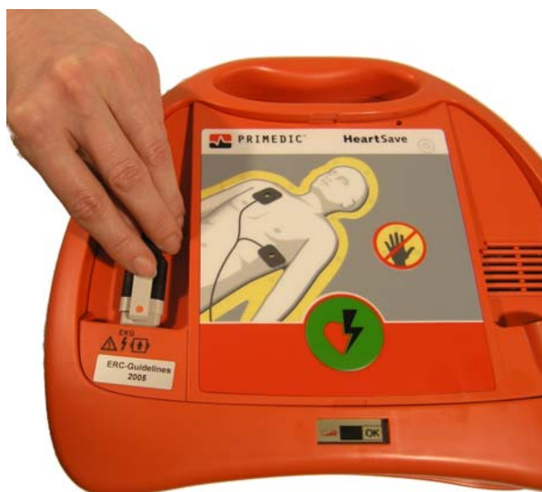
Fig. 12: Plugging in the electrode plugs
