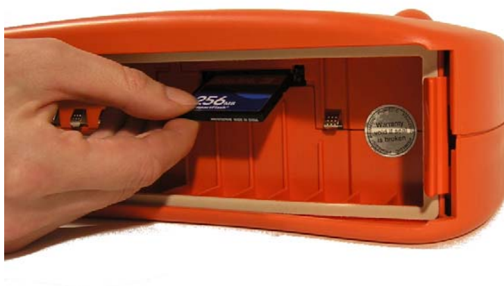
Fig. 7: Inserting / Changing the SaveCard
