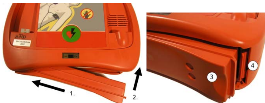
Fig. 8: Inserting the battery
